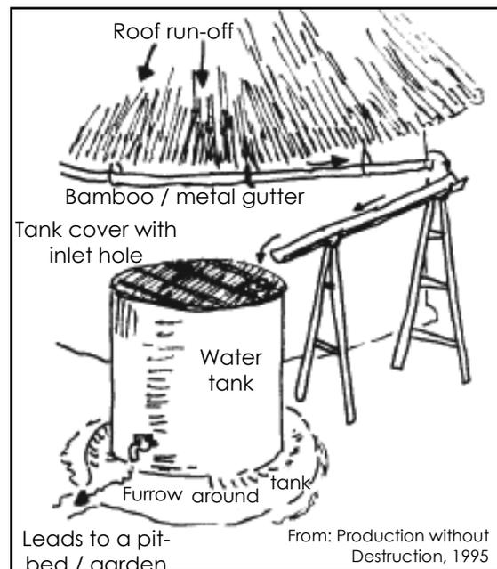
Collecting run-off from a thatched roof for use in the garden
