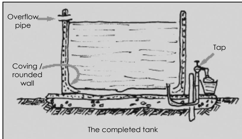
Then a small amount of water is put in the bottom of the tank and it is covered with black plastic or wet sacking for 7-10 days to cure. Break out any pipe fitting needed in the first few days. The tank needs to be filled slowly with water. Leave a shallow bit of water in the tank for about a week before filling it.
