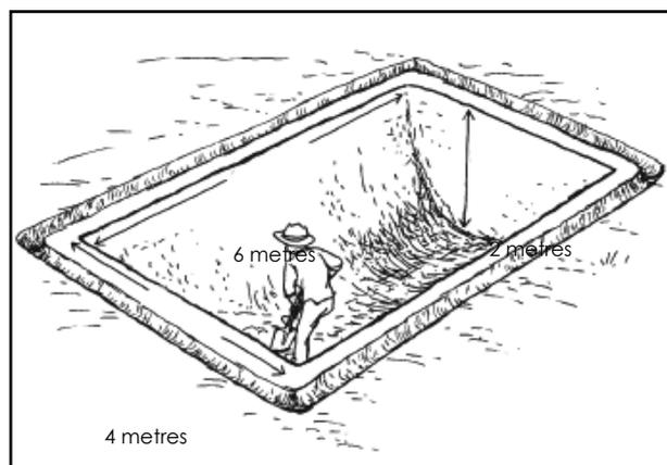
wide and 2 metres deep. There is a slight slope on the inner walls. This means that they are not dug straight down, but at a slight angle. When the pit is dug, stamp the soil inside the pit down, so that it is firm and smooth.
