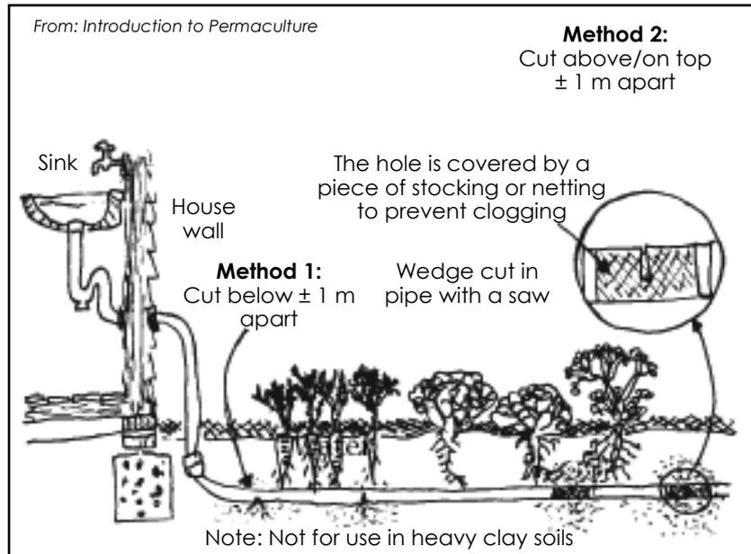
Below is another method of drip irrigation that you can use. Here we use pipes with small holes drilled or burned in the plastic. The pipes are laid on top of the ground and the whole bed (including the pipes) is covered with a good layer of mulch.
