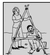
3 Now tie a piece of string onto the frame at the top. Attach the stone onto the end of the string. When you hold the frame up, the stone should hang just below the cross pole/bottom pole. Hold the A-frame upright on a level piece of ground/floor. Mark the place where the string hangs across the bottom pole. This should be close to the middle of the pole.
