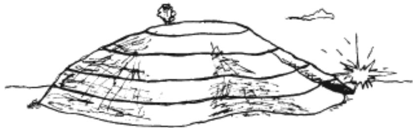
Contour lines drawn on a picture of a hill to show the areas that are level
