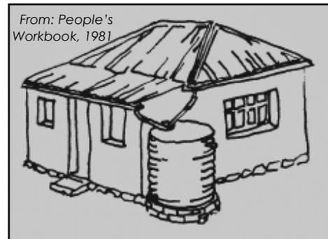
Water is channelled by gutters to the storage tank
